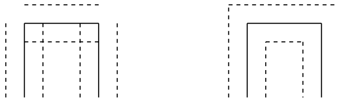
Figure 4: Construction of padding obstacles. Left: First step; drawing parallel lines. Right: Second step; clipping/joining them at intersections.
