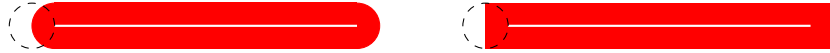
Figure 3: For a circular agent and line obstacle, Left: Exact configuration space obstacle, Right: Extended configuration space obstacle
